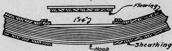
FIG. 2.—Cross-section through door, showing the construction of the door and the door opening for a wooden hoop silo.
