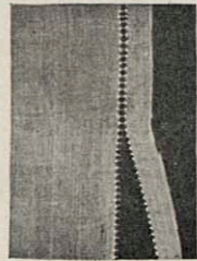
Ill. 249. Picot Edging Is Machine Hemstitching Cut Through the Center
