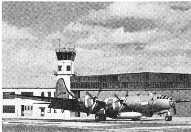
Pictured is one of four SB-29's, aerial search and rescue version of the Superfortress, on arrival at Wiesbaden Air Base. The planes are equipped with radar equipment and lifeboats. The main item, the A 3 li'eboat, is 30 feet long and can be dropped from 1,400 feet and remain upright. Its engine carries up to 200 gallons of gasoline and can be started and guided by radio. (USAFE photo)
